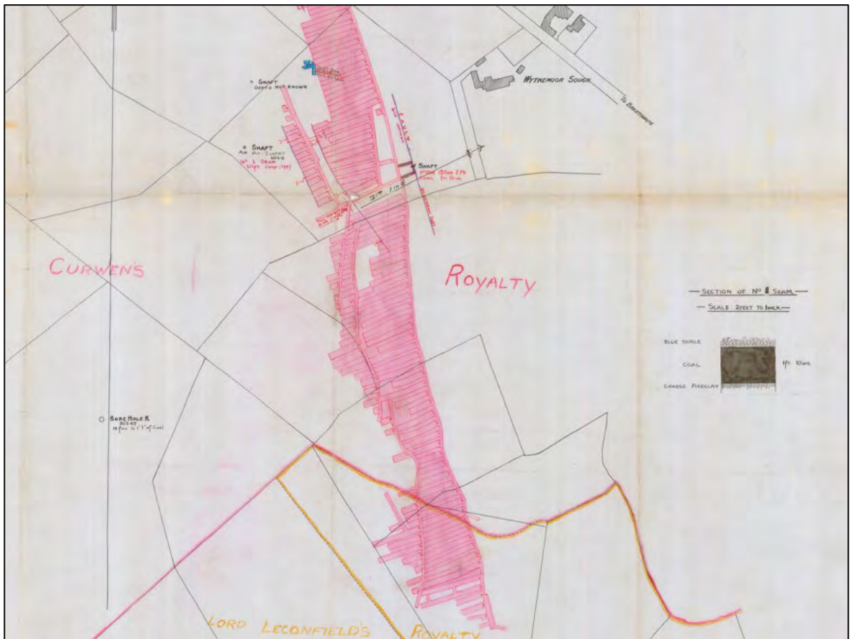
Plate 1: - Extract of mineplan showing extents of workings at the level of the No.1 Coal. Source: Coal Authority Mine Abandonment Plan 7837 (1 of 3). North arrow shown in top left corner, and cross section of worked seam included. Red line Boundary overlain.
